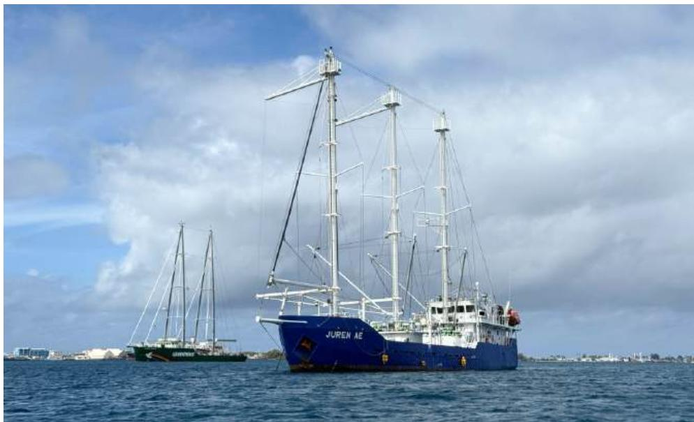
A key outcome of LCST is *Juren Ae*—a wind-powered cargo ship designed specifically for the pacific. Named after a traditional Marshallese canoe paddle, she blends heritage and innovation. The vessel reduces CO<sub>2</sub> emissions by up to 80% compared to conventional ships in the fleet, thanks to her sail system, solar panels, battery storage, and hybrid electric propulsion.
